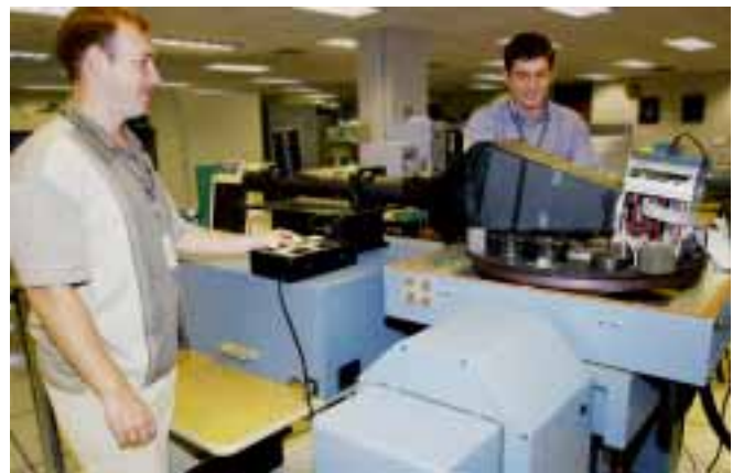
Tye Brady (left) and Clemens Tillier use star simulator to test sensitivity of active pixel sensor imager.
